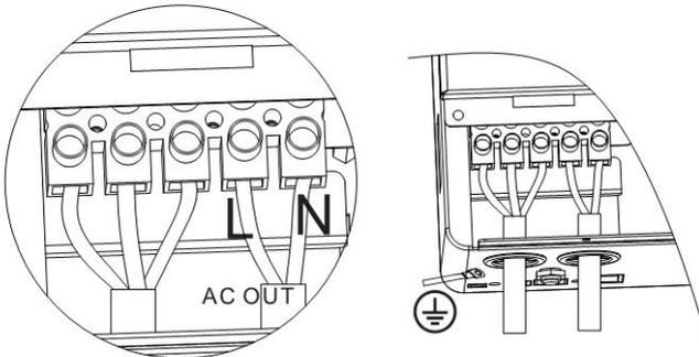
**Note:** The grounding wire shall be as thick as possible (cross-sectional area is not less than  $4\text{mm}^2$ ). The grounding point shall be as close as possible to the solar storage inverter. The shorter the grounding wire, the better.
