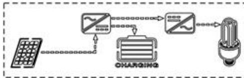
When the PV energy is less than the load, the battery replenishes power to the load.
