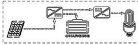
When the PV energy is less than the load, the battery replenish the power supply.
