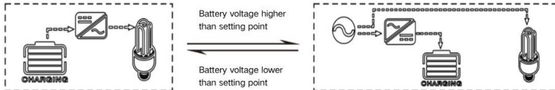
With BMS communication: when the battery SOC is lower than [61] setting items, switch to utility power supply and charging; when the battery SOC is higher than [62] setting items, switch to PV, battery to power the load.
