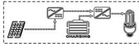
When PV is invalid, switch to mains power supply and charging. When PV is restored, switch back to PV and battery to power the load.
