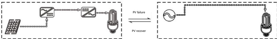
No BMS communication: when the battery voltage is lower than [04] setting item, switch to mains power supply and charging. When the battery voltage is higher than [05] setting item, switch back to PV and battery to supply power to the load.
