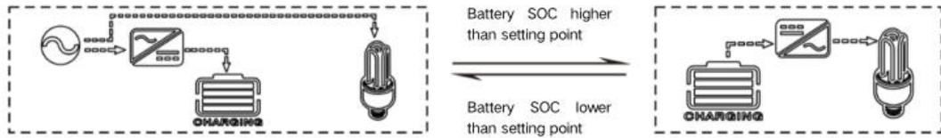
This mode maximizes the use of DC energy and is used in grid stable areas. Does not affect PV charging.
