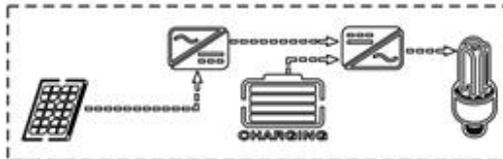
When the PV is ineffective, the battery power the load. Cycle the battery charge and discharge.
