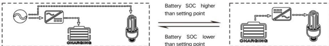
This model maximizes the use of solar energy while maintaining battery power and is suitable for areas with stable power grid.
