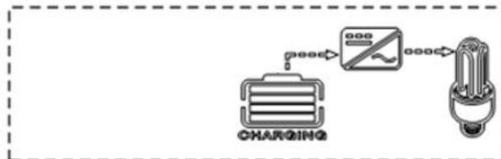
No BMS communication: When the battery voltage is lower than [04] setting item, switch to mains power supply and charging. When the battery voltage is higher than [05] setting item, switch to PV, battery to power the load.
