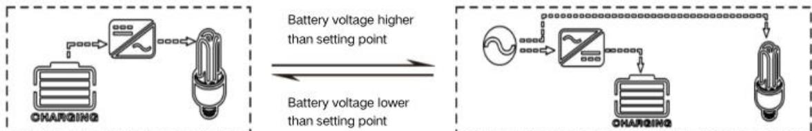
With BMS communication: when the battery SOC is lower than the [61] setting item, switch to utility power supply and charging; when the battery SOC is higher than the [62] setting item, switch to PV, battery to power the load.
